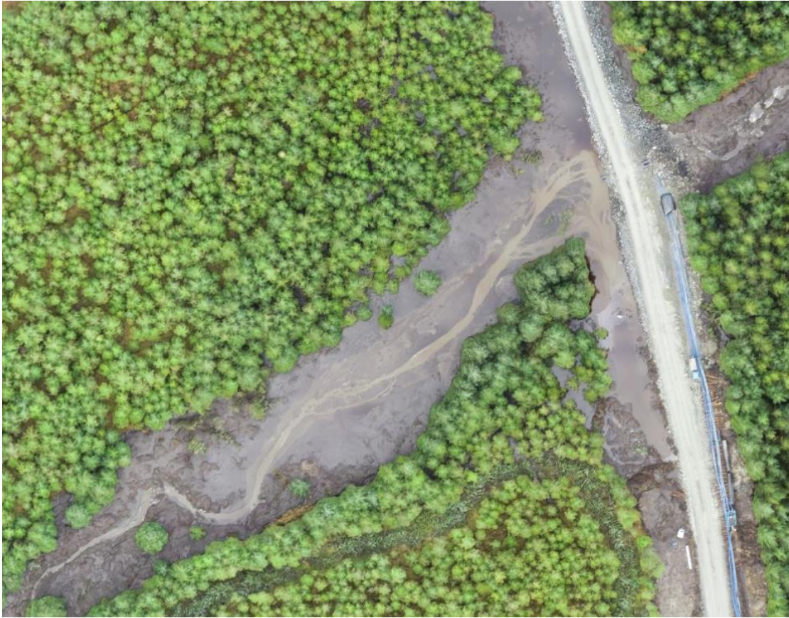
Figure 5.3 Aerial image of water and peat impoundment area upstream of Wall 1 showing large volumes of impounded peat and clearly identifiable channel for water reaching Wall 1
