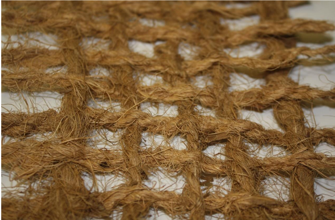
Figure 5.9 CoriMesh biodegradable woven coconut fibre used on bare surfaces to prevent erosion and promote revegetation
